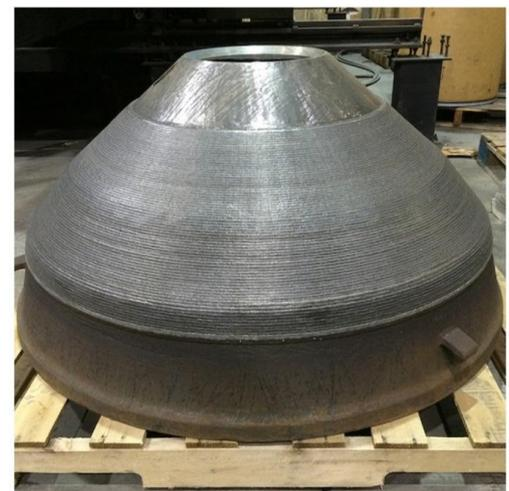
In addition, random and/or systematic variations on wires and hardfacing welding procedures result in finished products with large discrepancies in performance. Environmental costs due to excessive use of highly polluting Chromium (Cr) are also a big concern, as well as the increasingly strict environmental regulations that push for lean welding consumables.
